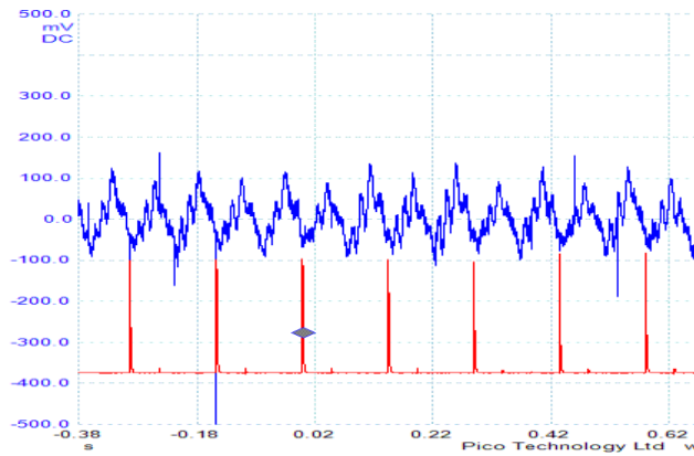
Crankcase Test – Good Cylinders Diesel
