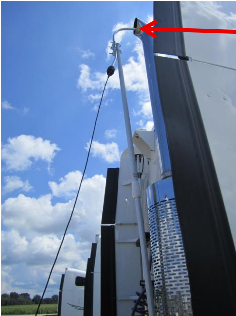
Shepherd's hook exhaust sensor on telescopic pole inserted into the vertical exhaust.
